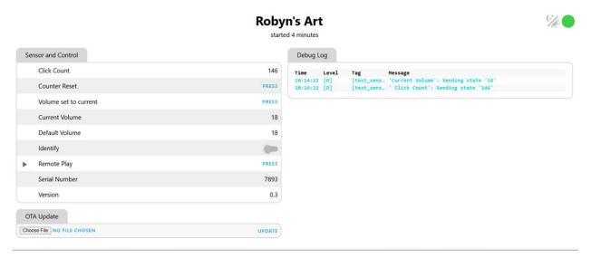
**Click Count:** The number of times the 'Start' button has been pressed and the recording played since the counter was reset. The counter is persistent across reboots and firmware upgrades.
