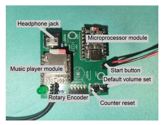
The AMP2 is a small, self-contained media player designed to provide audio descriptions to accompany a public art display. The AMP2 is intuitive and easy to use for all patrons, including those with low vision. Operation is controlled with a single large, high visibility button on the front panel, and a volume control on the bottom of the unit. Headphones and power cables are captive when the AMP2 is mounted, preventing casual theft.
