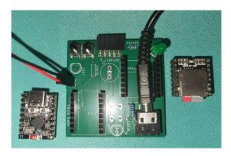
Connect power to the AMP2. Connect a power cable to the USB-C connector directly on the ESP32 microprocessor module.
